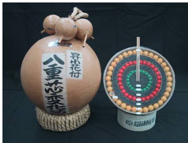
Figure 2 – Model of fireworks shell (left) and its half section one (right).
